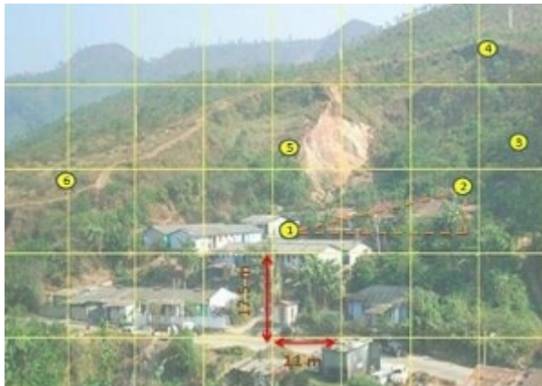
Fig. 6. Deep Earth Probe Deployment Locations at the Anthoniari Colony Site, Munnar, Kerala, India
