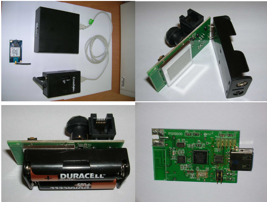
Fig. 7. Gateway based on miniPC, Mote board and base station
