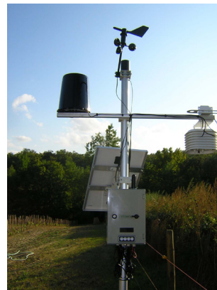
(b) VineSense GPRS Gateway with Weather Sensors
