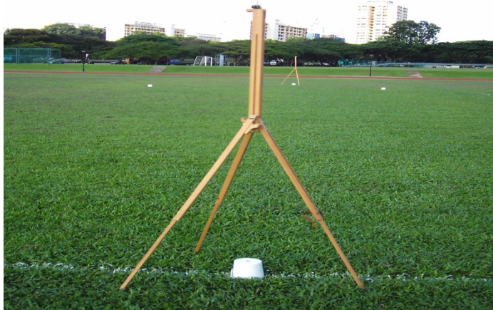
Fig. 14. Reference nodes mounted 190 cm above ground; sensor nodes are mounted on plastic pots 12 cm above ground level.
