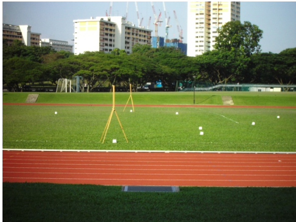
Fig. 12. ALS experiment in an obstacle free environment – the experiment was carried out in a 30m×30m region in a soccer field. There were no obstacles present inside the region.
